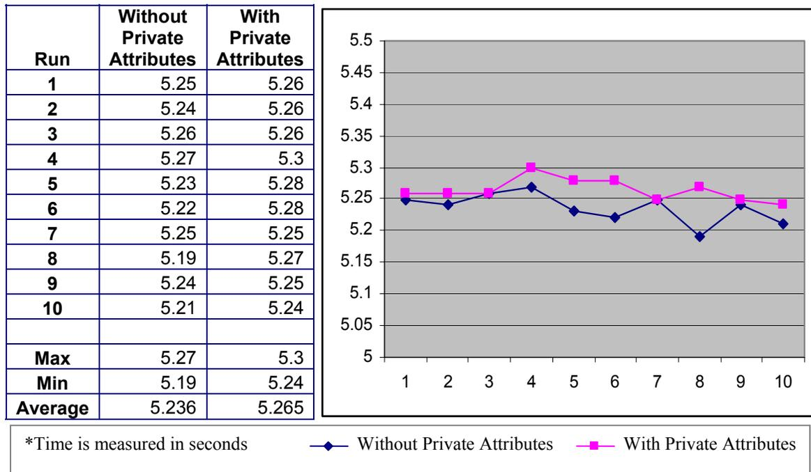
**Figure 17 – The Cost of Private Attributes in Trust Negotiation.** The graph and data show the contrast between identical scenarios involving the same number of rounds of trust negotiation; one test of trust negotiation over HTTP with private attribute support and the other without, showing the cost to be negligible.
