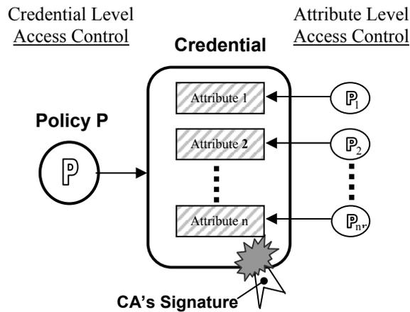
**Figure 6 – Levels of Access Control.** Policy P is an access-control policy that protects a sensitive credential, and constitutes credential level access-control. P<sub>1</sub> – P<sub>n</sub> are policies independently govern access to each attribute and constitute attribute-level access control.
