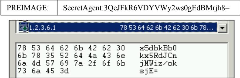
**Figure 11 – A View of the Private Attribute Pre-image and its associated digest.** The example certificate’s extension contains a private attribute digest visible in the Windows Certificate Viewer. The associated pre-image used to originally create the digest contains the actual attribute value “SecretAgent” followed by a separator and 28 bytes of random data.
