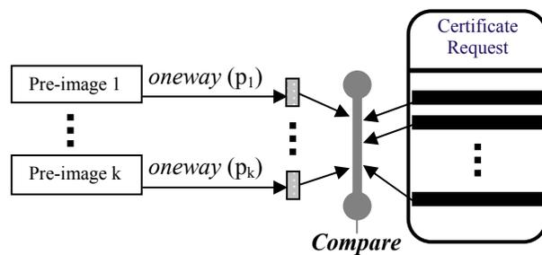
**Figure 9 – The CA’s Verification Process.** Taking the pre-images sent by the certificate requestor  $p_1 \dots p_k$ , the CA calls the specified one-way function on them and compares each result to the corresponding private attribute digest within the credential verifying the credential’s sensitive attributes.
